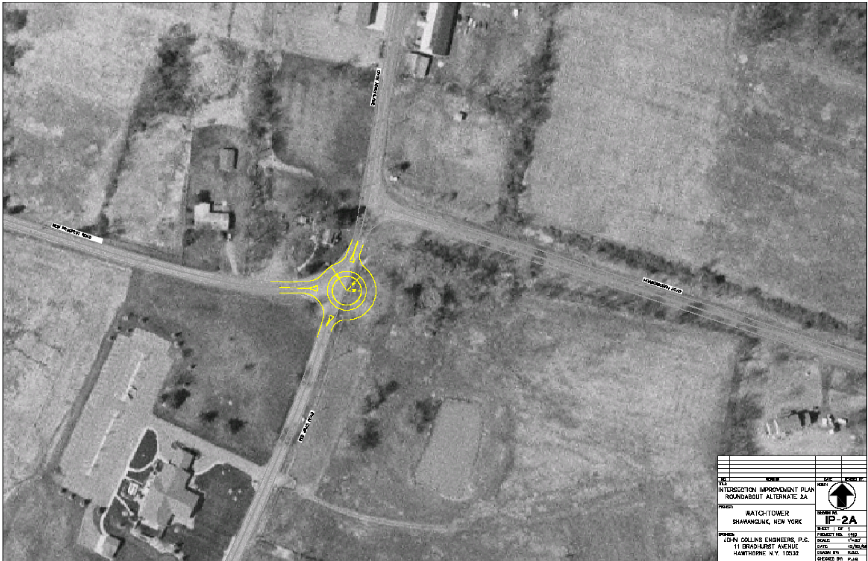
Figure III.G-5 Intersection Improvement Plan Roundabout Alternate 2A (IP-2A)
